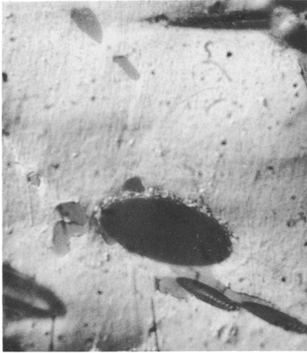
Figure 8 F-M interface failed during creeping. \times 1100 .
